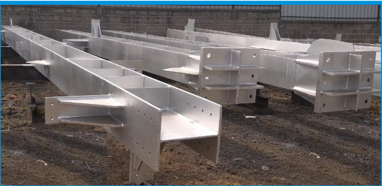
COLUMNS WITH BLASTING AND PAINTING
